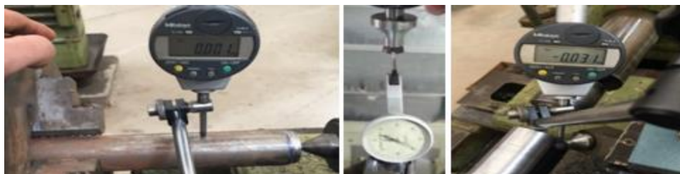
Fig. 4 Multiple Setup for machining processes, Preparation of specimens and install the SPRT and adjust run out using dial indicators
