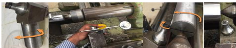
Fig. 5 SPRT Set-up, Install the tool and tool holder and adjust the tool at a machining center for different tilting angles.
