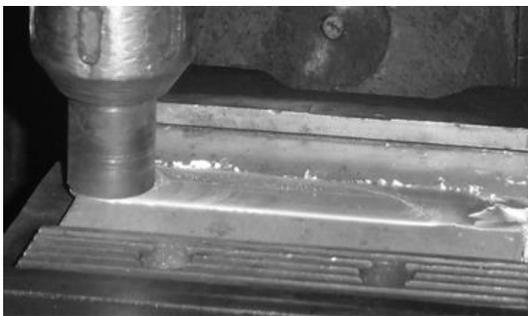
Fig (1). The FSW process.
