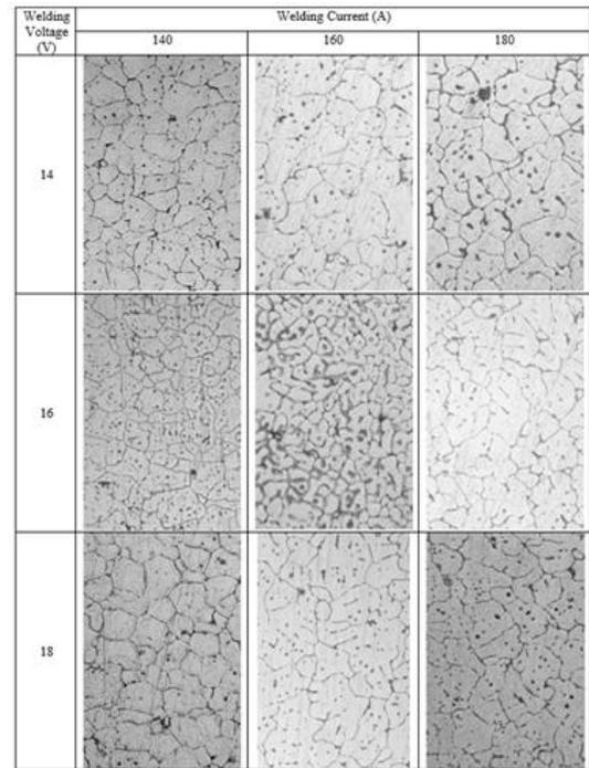
Fig (7). Microstructure at the center of FZ for AA6061-O samples MIG welded using different voltages and currents ( $\times 100$ ).
