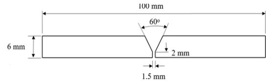
Fig (2). V-butt joint configuration of MIG welding samples.
