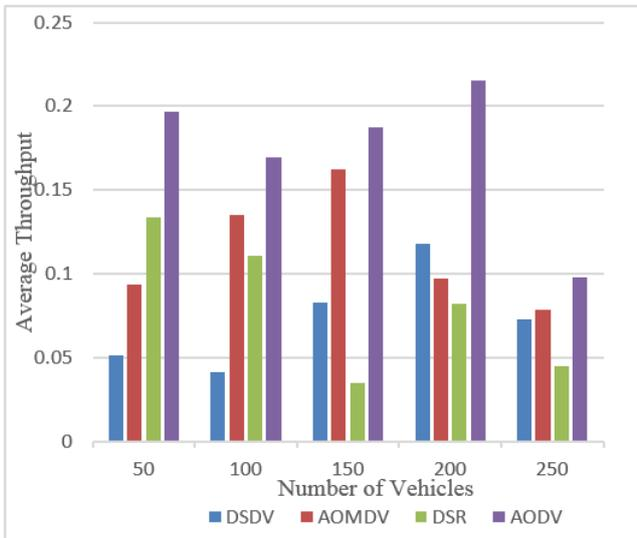
Figure 3 Average throughput ratio VS. Number of vehicles for (AOMDV, DSDV, DSR and AODV)
