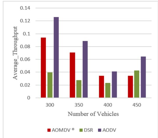
Figure 4 Average throughput ratio VS. Number of vehicles for (AOMDV, DSR and AODV)
