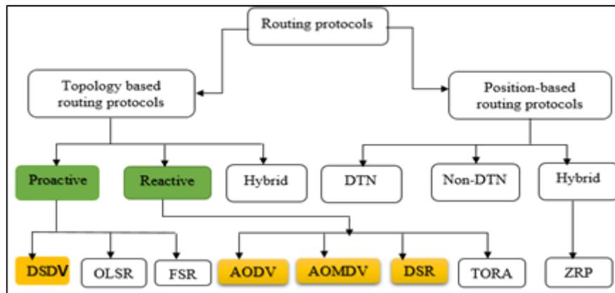
Figure 2 VANET Routing Protocols [3]
