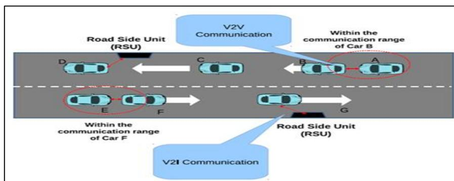
Figure 1 Creating an Ad-hoc Network using Vehicles (VANETs) [1]
