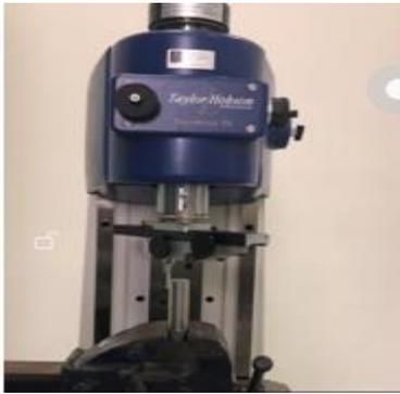
Fig. 5. Photograph of Taylor-Hobson talysond 73 roundness tester.
