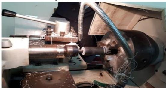
Fig. 3. The turning of epoxy/BN nanocomposites
