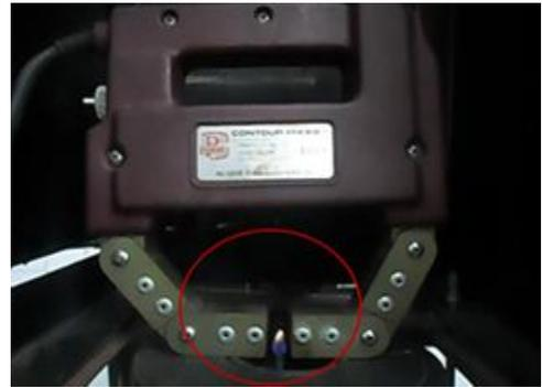
Fig (1) : The electromagnetic yoke coil placed around the candle flame.
