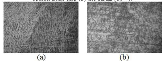
Fig 7. Microstructure of AISI 316 stainless steel region welded using E312-17 electrode by SMAW; (a) the fusion zone and (b) the HAZ (10 ×).
