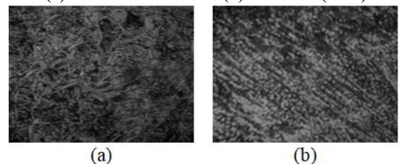
Fig 9. Microstructure of AISI 316 stainless steel region welded using ER312 electrode by GTAW; (a) the fusion zone and (b) the HAZ (10 ×).
