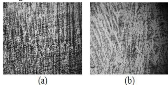
Fig 2. Microstructure of AISI 304 stainless steel region welded using E308L-16 electrode by SMAW; (a) the fusion zone and (b) the HAZ (10×).
