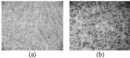
Fig 3. Microstructure of AISI 304 stainless steel region welded using E312-17 electrode by SMAW; (a) the fusion zone and (b) the HAZ (10 ×).
