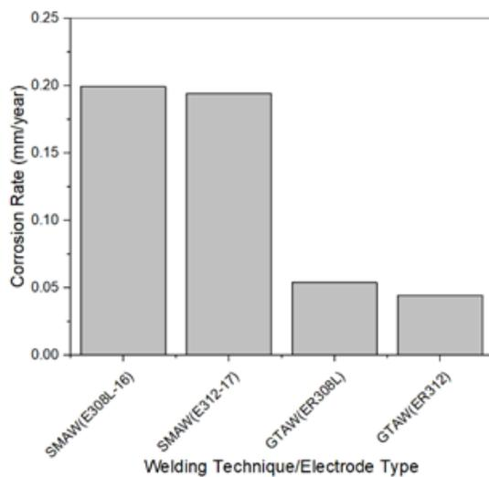
Fig 10. Variation of the corrosion rate at the center of the fusion zone with the welding technique and electrode type for AISI 304 stainless steel welded joints.
