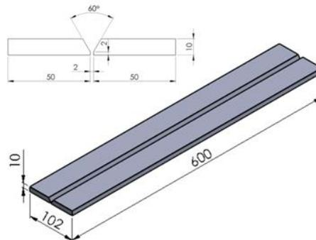
Fig 1. The welded joint configurations (dimensions in mm).
