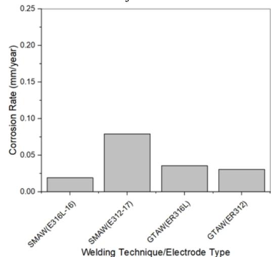
Fig 3.1. Variation of the corrosion rate at the center of the fusion zone with the welding technique and electrode type for AISI 316 stainless steel welded joints.
