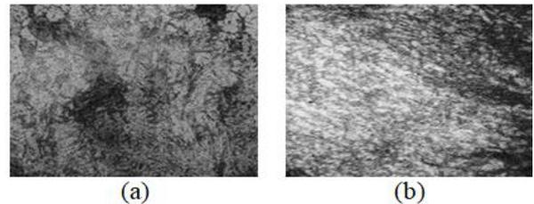
Fig 6. Microstructure of AISI 316 stainless steel region welded using E316L-16 electrode by SMAW; (a) the fusion zone and (b) the HAZ (10 ×).
