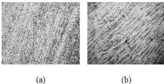
Fig 5. Microstructure of AISI 304 stainless steel region welded using ER312 electrode by GTAW; (a) the fusion zone and (b) the HAZ (10 ×).
