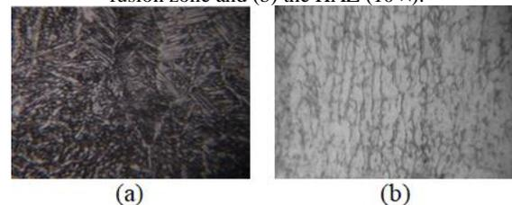
Fig 8. Microstructure of AISI 316 stainless steel region welded using ER316L electrode by GTAW; (a) the fusion zone and (b) the HAZ (10 ×).
