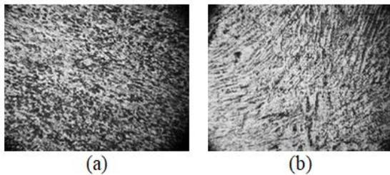
Fig 4. Microstructure of AISI 304 stainless steel region welded using ER308L electrode by GTAW; (a) the fusion zone and (b) the HAZ (10 ×).
