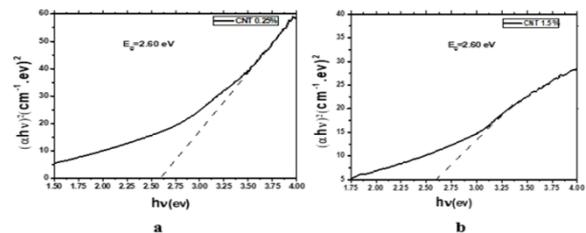
Fig 3. Variation of  $(\alpha h\nu)^2$  with photon energy  $h\nu$  for epoxy/MWCNTs nanocomposites containing (a) 0.25 wt.-% and (b) 1.5 wt.-% of MWCNTs nanofillers.
