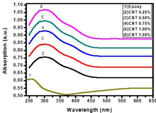
Fig 2. Optical absorption spectra of epoxy/MWCNTs nanocomposites
