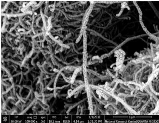
Fig 1. SEM micrographs of the MWCNTs nanofillers.
