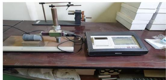
Fig 4. Surface roughness measurement device (MitutoyoSurftest SJ-310)
